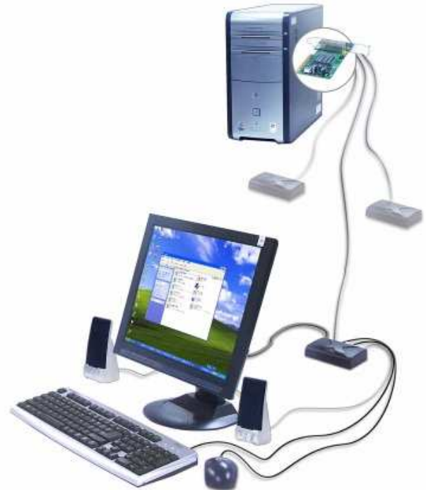
The X300 kit is easy to install and includes one PCI card and three small access terminals
