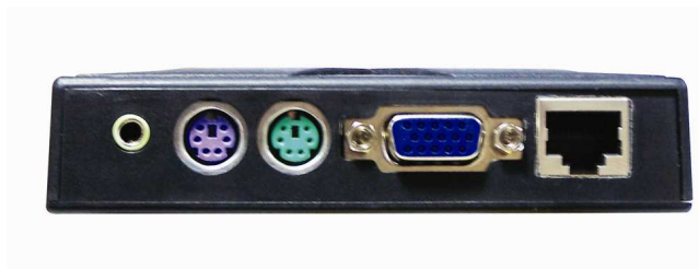
Standard PS/2 keyboard, PS/2 mouse, VGA and audio ports connect to user peripherals
